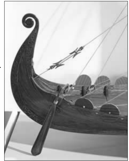
The rudder was attached near the stern of the boat on the starboard (Steer-board) side.
